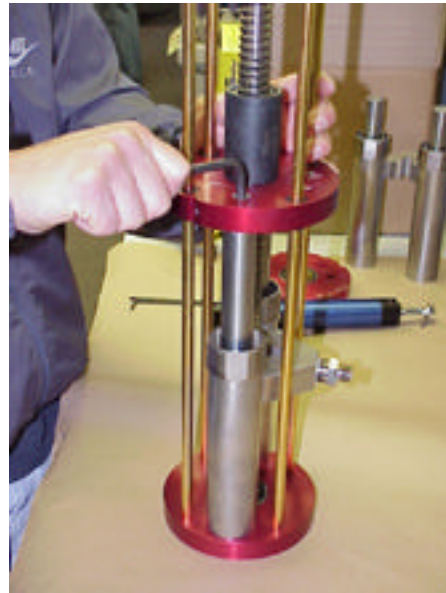
Remove two 5/16-24 SHCS that connect the Center Plate to the two LDP Rods.
