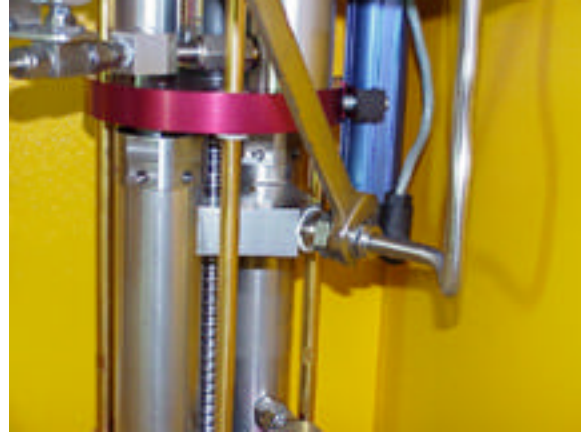
Detach the SS hard line from the lower cylinder Manifold. It will be necessary to loosen the nut on the other end of the tube connected to the Cross Over Valve.
