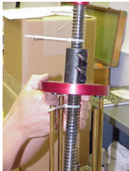
Lift the Center Plate Ball Screw Assembly off the Linear Shafts and set aside.
