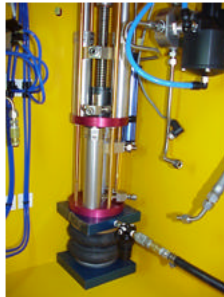
Center the Pump Lift under LDP and raise it until it seats against the bottom of the pump.
