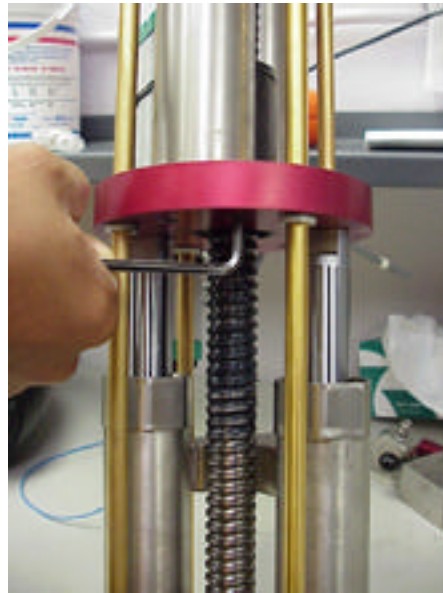
Remove four ¼-20 SHCS connecting Upper Cylinders to the Center Plate.
