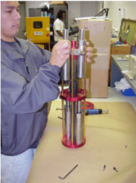
Remove the Upper Cylinder Set and set aside.
