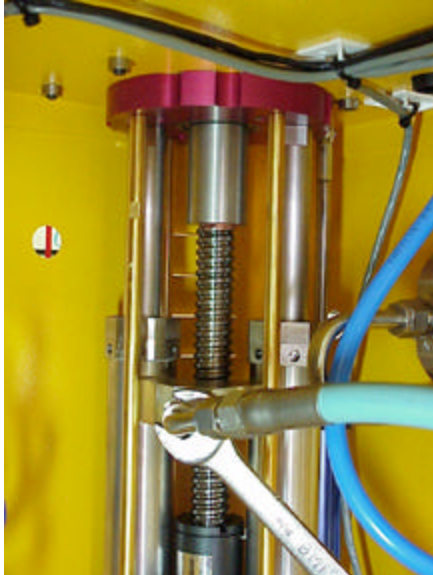
Detach the Flex Hose compression nut from the upper cylinder manifold.
