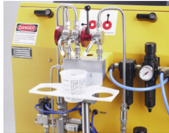
Ratio Check Station used as a Fill Station
