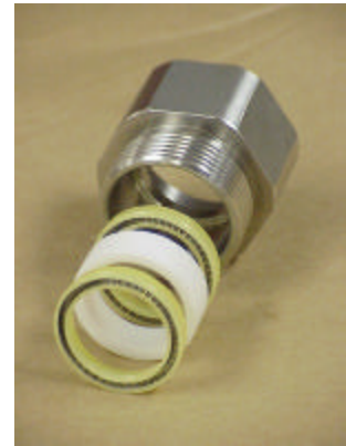
Install New Seal & Bearing
