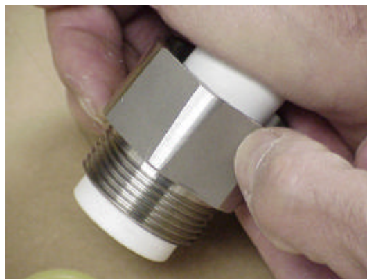
Push Out Old Bearing and Seal/s
